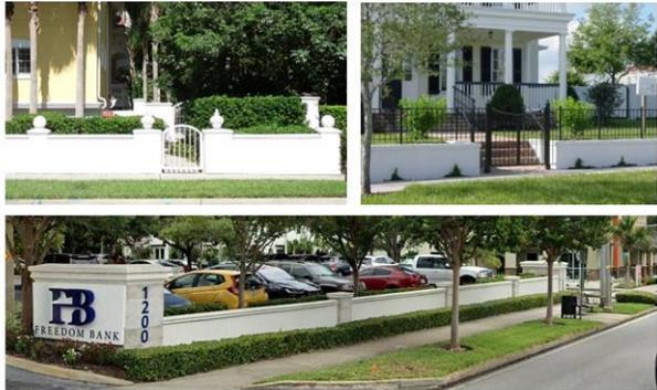
2.5 feet to 5 feet. The portion above 2.5 feet shall be transparent (e.g., wrought iron or similar material). Street walls shall have columns/posts (one foot by one foot minimum) spaced every 24 feet.
